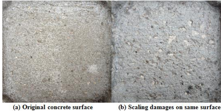
Figure 2. Typical Scaling Damage
