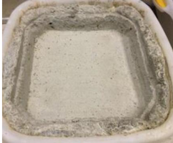
Figure 14. Concrete slab for salt scaling evaluation
