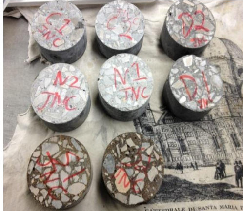
Figure 9. 2-in circular disks for water absorption test
