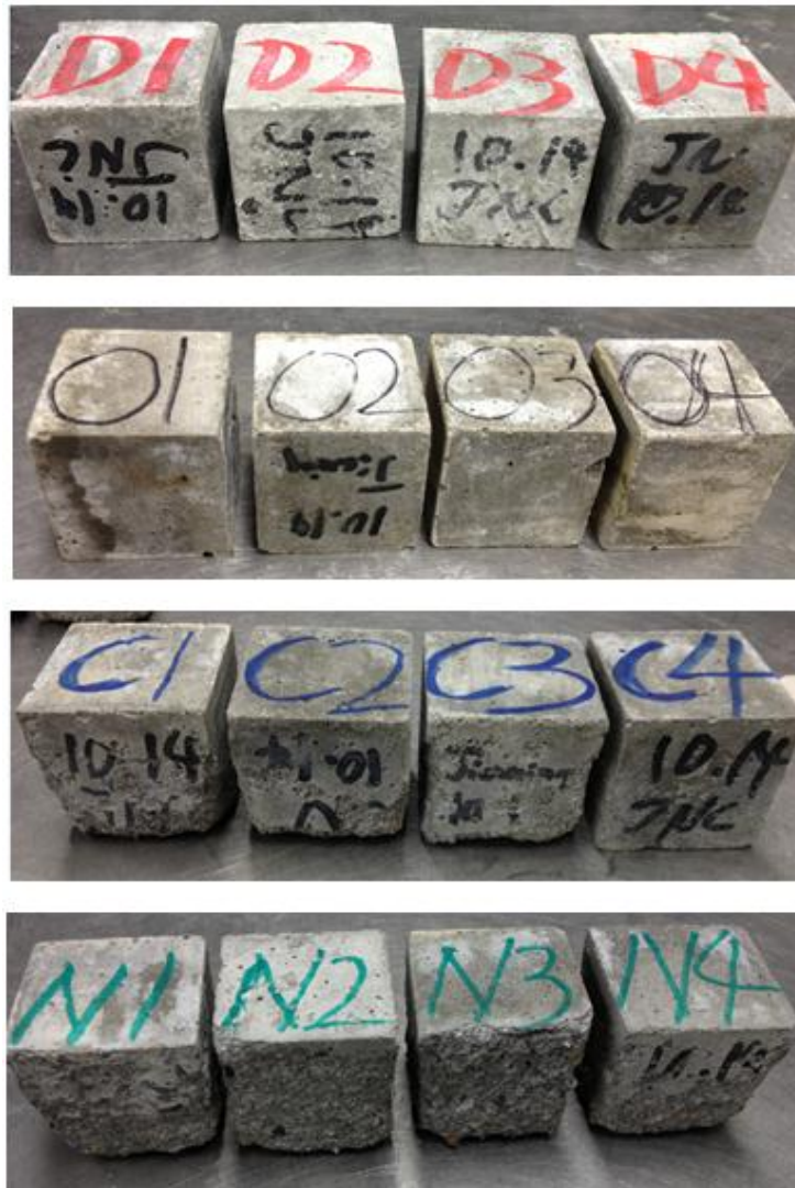
Figure 24. Cubes with surface materials removed after 10 cycles
