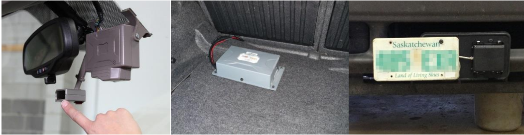
Figure 3.5 Head unit, main unit, and front radar used in Canada naturalistic driving Study (Hankey, 2014)
