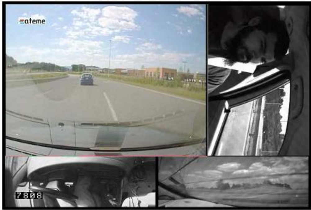
Figure 3.9 Four camera views from the SHRP2 data acquisition system: forward view (upper left), in-cabin driver face view (upper right), instrument panel view (bottom left), rear view (bottom right). (The driver in the picture is not experimental participant and just for demonstration purpose only) (Dingus et al., 2014)
