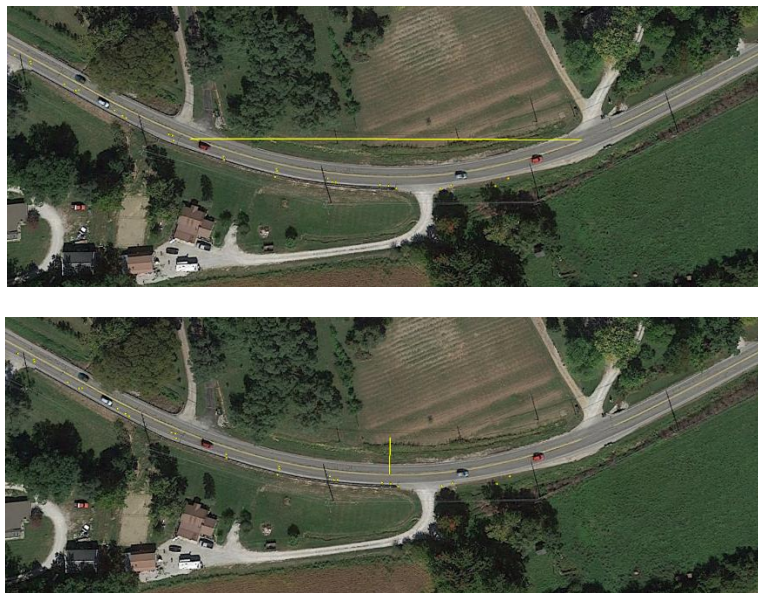
Figure 4.3 Curve radius measurement from chord length and offset distance (Google Map, 2015)
