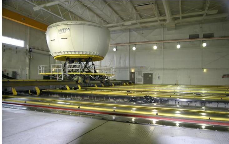
Figure 1.3 National advanced driving simulator at University of Iowa (National Advanced Driving Simulator, 2015)
