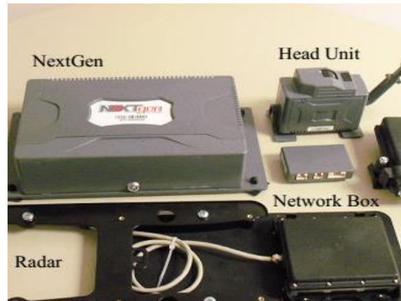
Figure 3.7 Data acquisition system components used in the SHRP2 NDS (including NextGen, Head Unit, Radar, Network Box, Radar Interface Box (Dingus et al., 2014)
