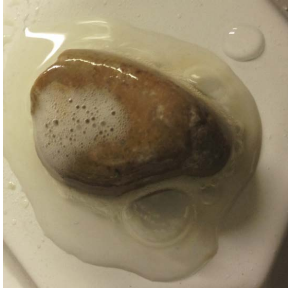
Figure 6: Carbonate Aggregate Surface React with Acid Solution
