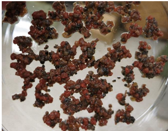
Figure B.3. Granules in UASB #2 reactor.
