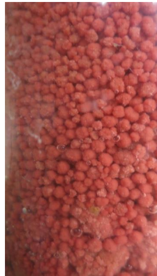
Figure B.1. Mature anammox granules in UASB #1 reactor on Day 66 under steady state operating condition (Influent \text{NH}_4^+\text{-N} =35 mM).
