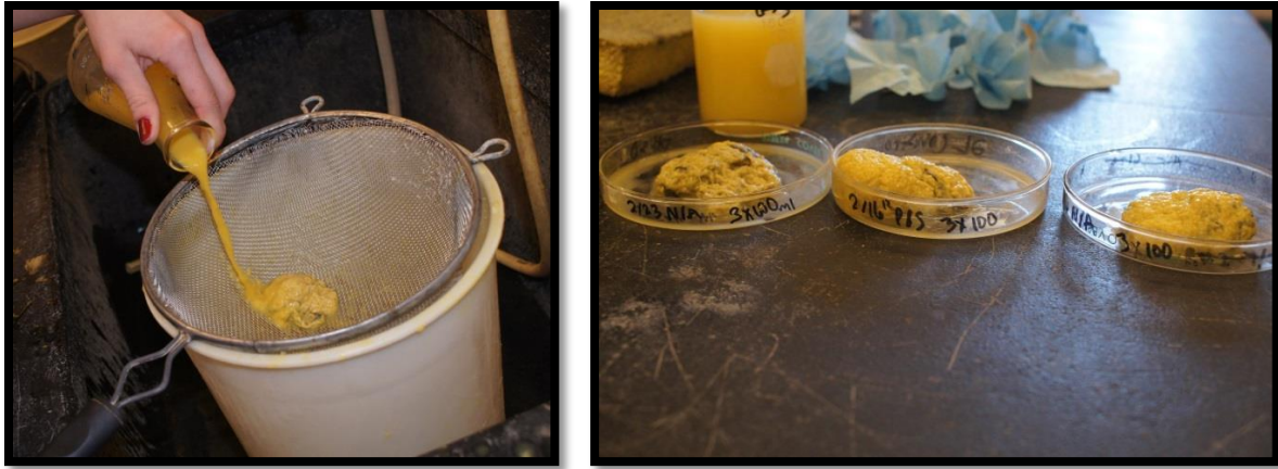
Figure 3.3. Harvesting of fungal biomass. Straining fungal biomass from thin stillage (left). Figure 3.4. Dewatered fungal biomass placed in petri dishes (right).
