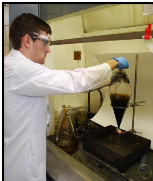
Figure 4.6. HTL sample with methylene chloride being poured into a Buchner funnel for % char determination (left)
