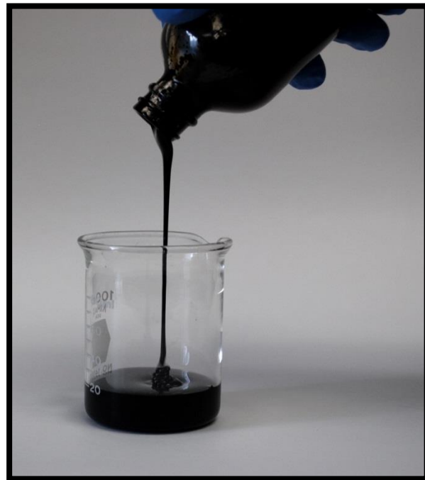
Figure 4.5. Bio-crude oil sample from HTL 1 test (right)
