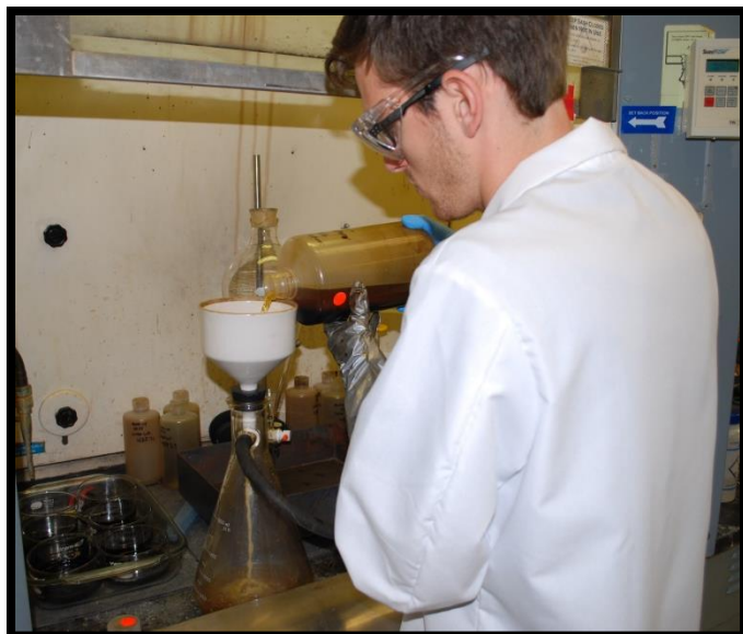
Figure 4.6. HTL sample with methylene chloride being poured into a Buchner funnel for % char determination (left)
