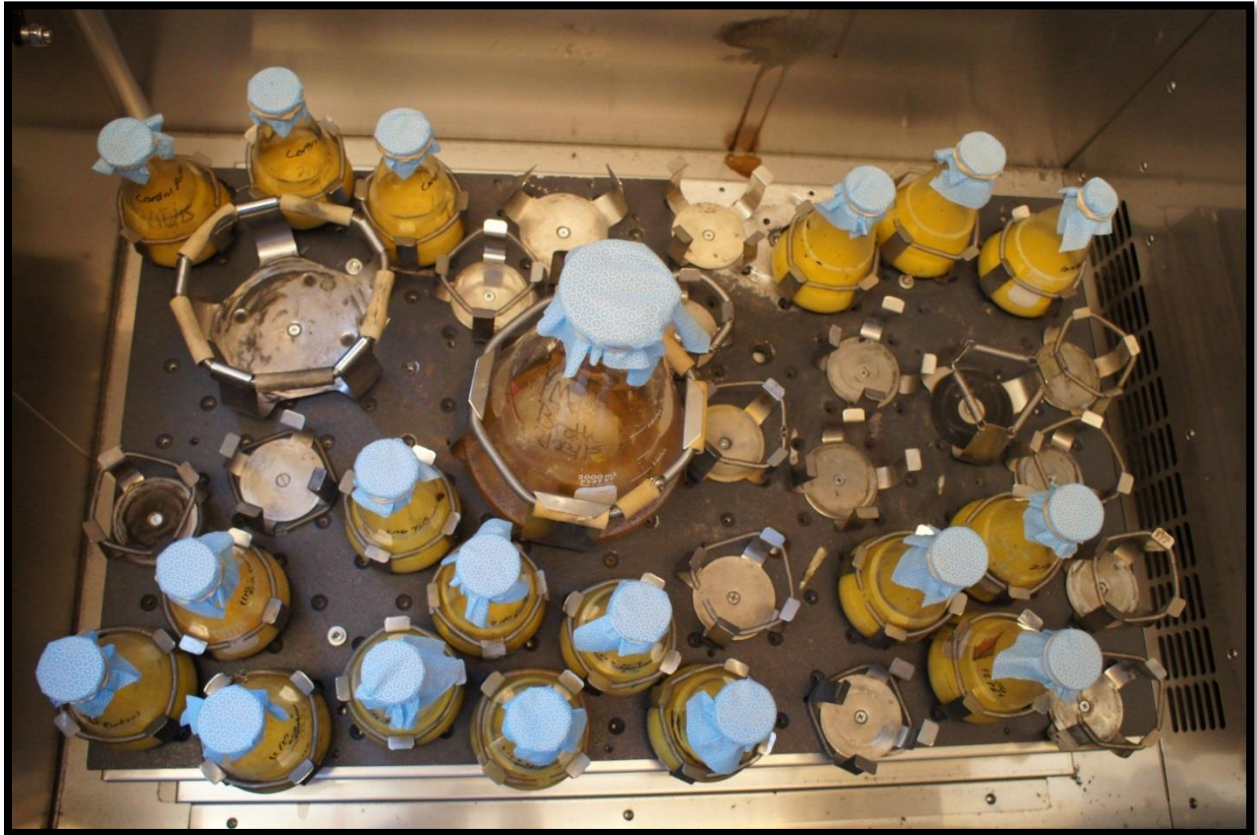
Figure 3.1. 250mL-scale reactors and 2 L flask of YM broth in shaker incubator
