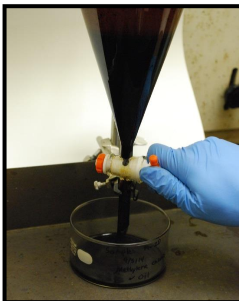
Figure 4.8. Stratification in the separatory funnel of HTL sample aqueous fraction (top layer) and methylene chloride soluble fraction (bottom layer) (left)
