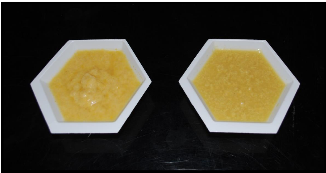
Figure 4.1. 5% fungal slurry course mixed (left), high shear mixed (right). Fungal slurry prepared 7/2/14.
