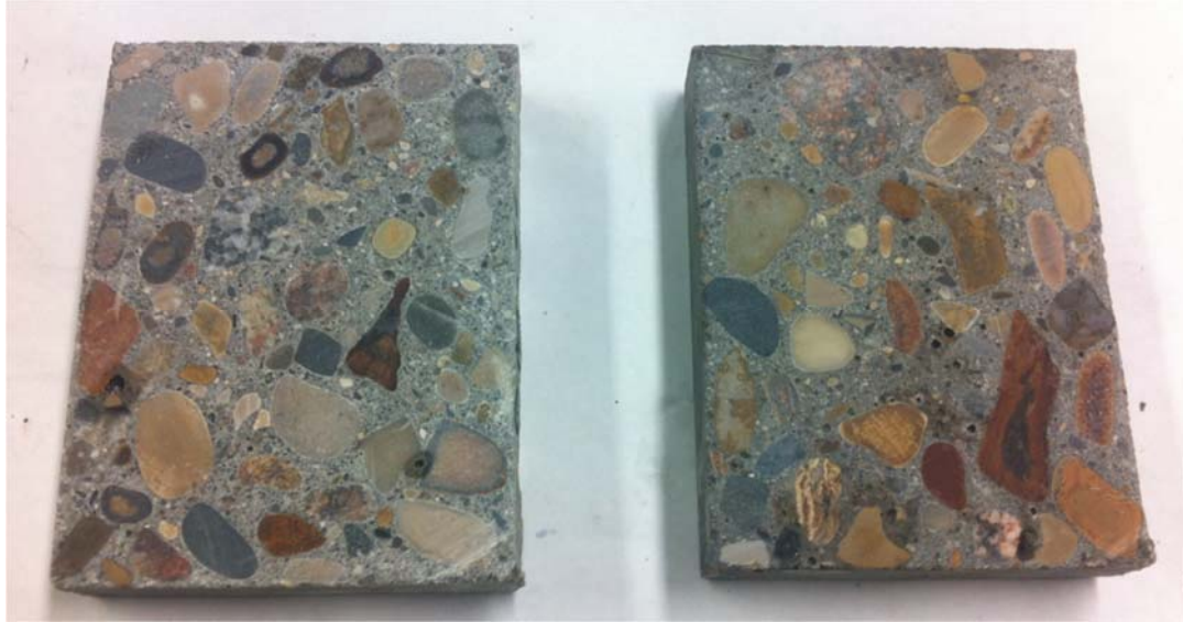
Figure 20. Concrete slices before soaking
