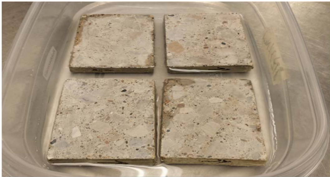
Figure 21. Slices immersed in salt solution
