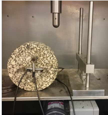
Figure 6.4 IDT dynamic modulus testing setup.
