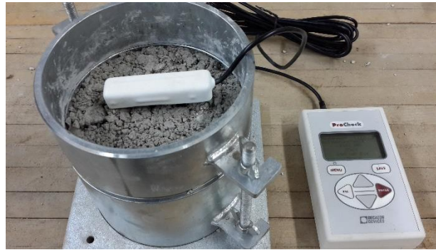
Figure 3.3 Laboratory dielectric constant measurement on a compacted crushed limestone sample
