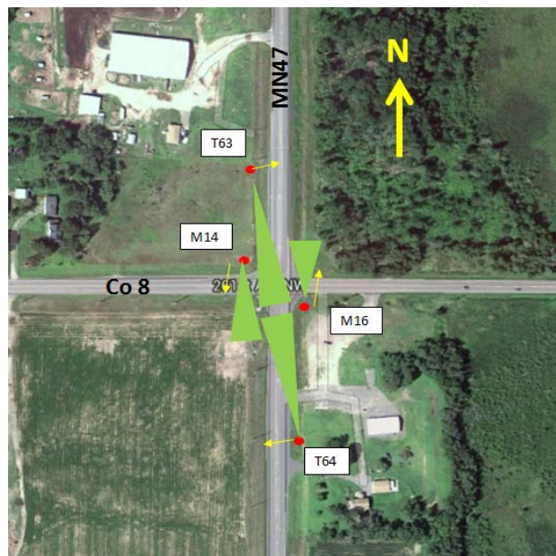
Figure 7: Isanti treatment intersection camera layout
