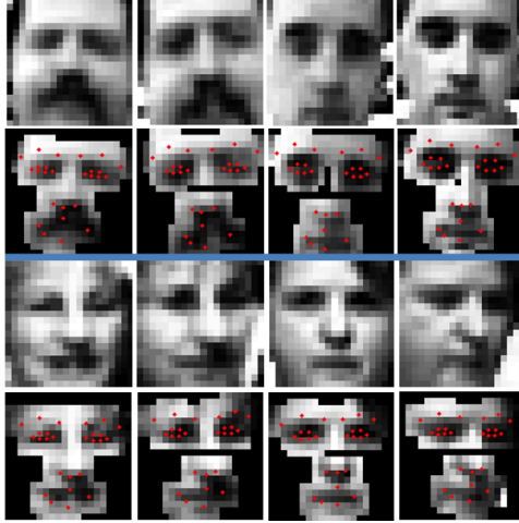
Figure 3.2: For illustration purposes, we visualize the single-scale patch image for the MBGC dataset by assembling all 5 \times 5 -pixel patches centered at 26 facial landmarks points together.
