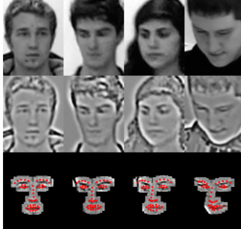
Figure 4.2: The first row shows the original image before preprocessing. The second row is the image after illumination normalization. The final row demonstrates the facial landmarks and patches used in this chapter.
