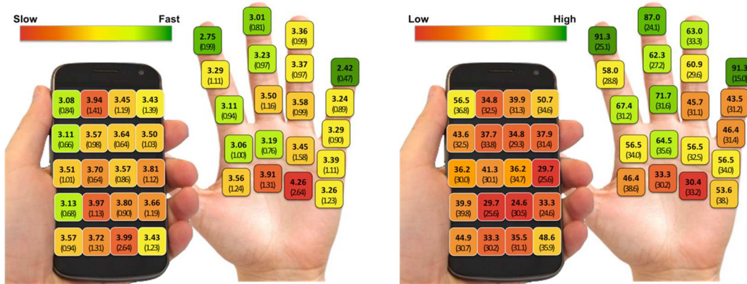
Figure 5.5. Heat maps for average selection time (left; sec.), and first contact point accuracy (right; %) per target in the pointing task, averaged across participants (with SD in parentheses) ( N = 23 ). The fingertips resulted in particularly strong performance results.
