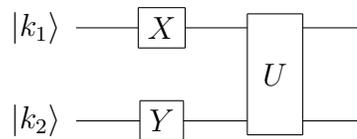
Figure 1.1: Example of a Quantum Circuit
