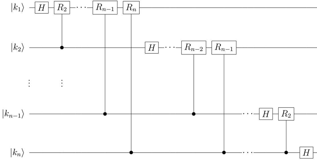
Figure A.1: Circuit Decomposition for Cyclic QFT
