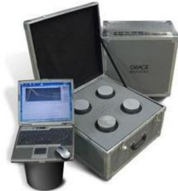
Figure 3. Calorimetry test equipment for heat of hydration of concrete.
