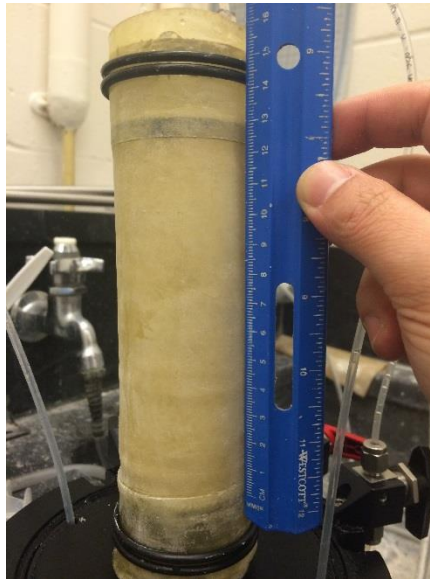
Figure 6.5 A sand specimen prepared by moisture tamping method
