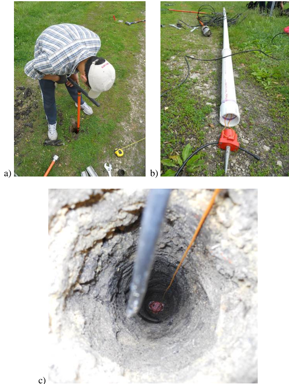
Figure 6.10 Borehole geophone preparation for MIBS field testing: (a) drilling borehole by hand-auger, (b) PVC pipe insertion device for borehole geophone, and (c) borehole geophone coupled to bottom of borehole by ground spike.
