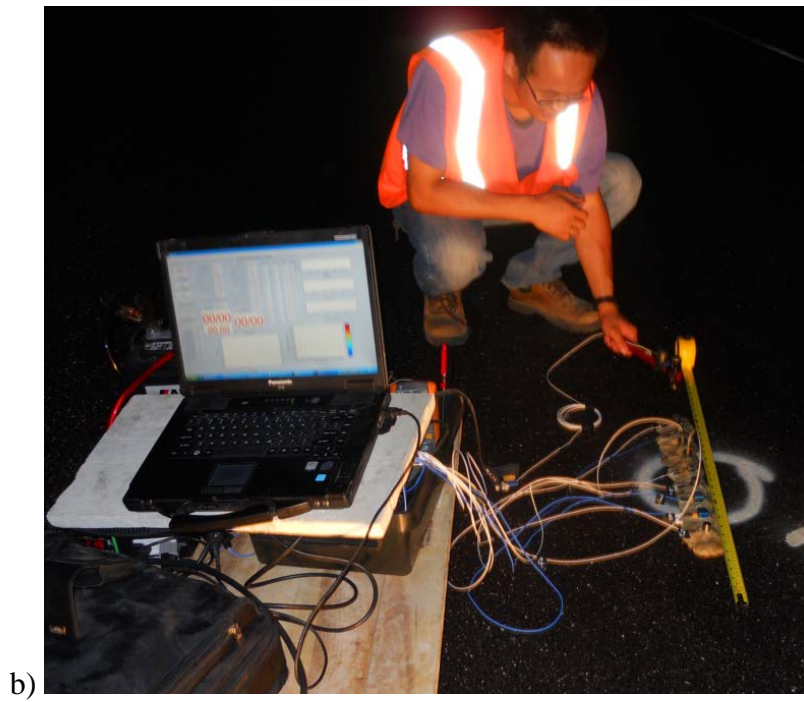
Figure 5.9 Typical field setups for pavement tests: (a) MSOR and (b) MASW.
