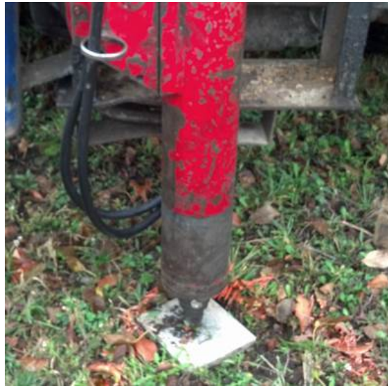
Figure 6.24 Preliminary MMSW-SPT test: a) SPT drill rig and geophone layout, b) SPT hammer impacting aluminum plate on the soil surface.
