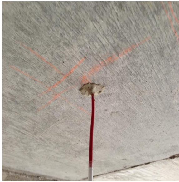
Figure 21. Thermistors at the bottom of deck
