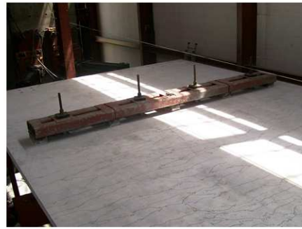
c. Flexural cracking across the entire deck width
