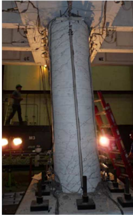
a. Column at 180 mm lateral displacement (displacement ductility +10.0)
