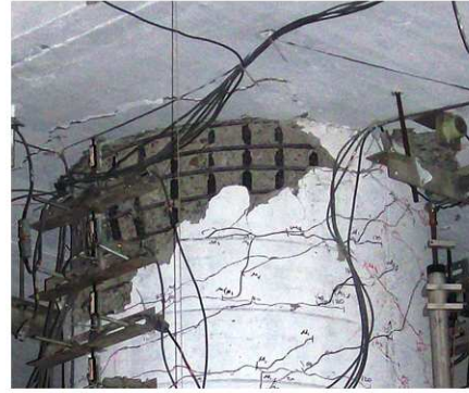
b. Buckled bars in the column top plastic hinge region
