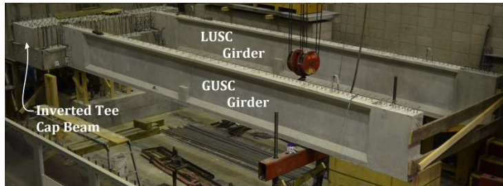
b. Girders prior to diaphragm and deck placement
