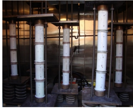
Loaded specimens for creep tests
