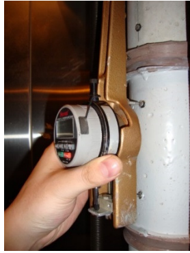
Strain measurement using the DEMEC gage
