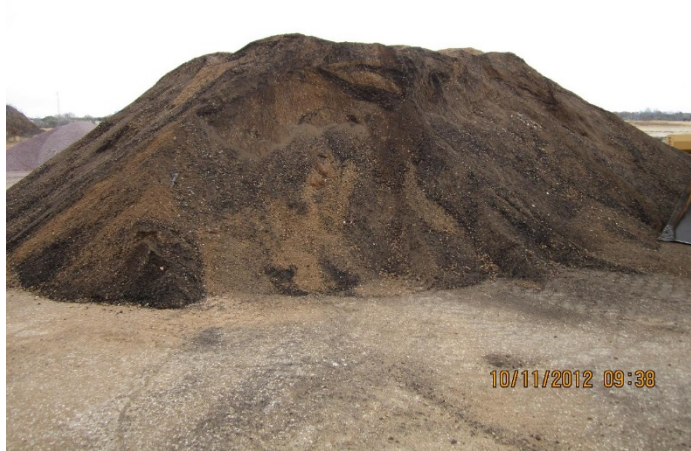
Figure 9 Shingles and Gravel Stockpile (Thomas J. Wood et al. 2014)
