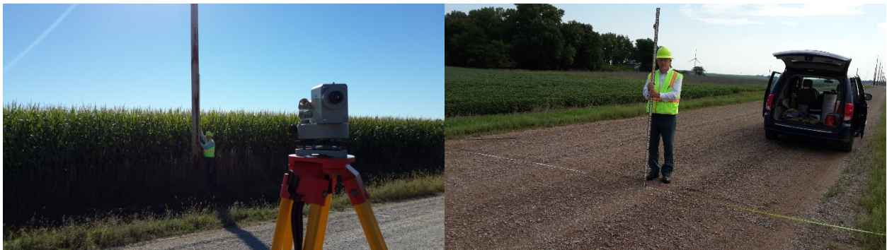
Figure 17 Automatic Level for Cross-Section Elevation Reading (Photo by the Author)
