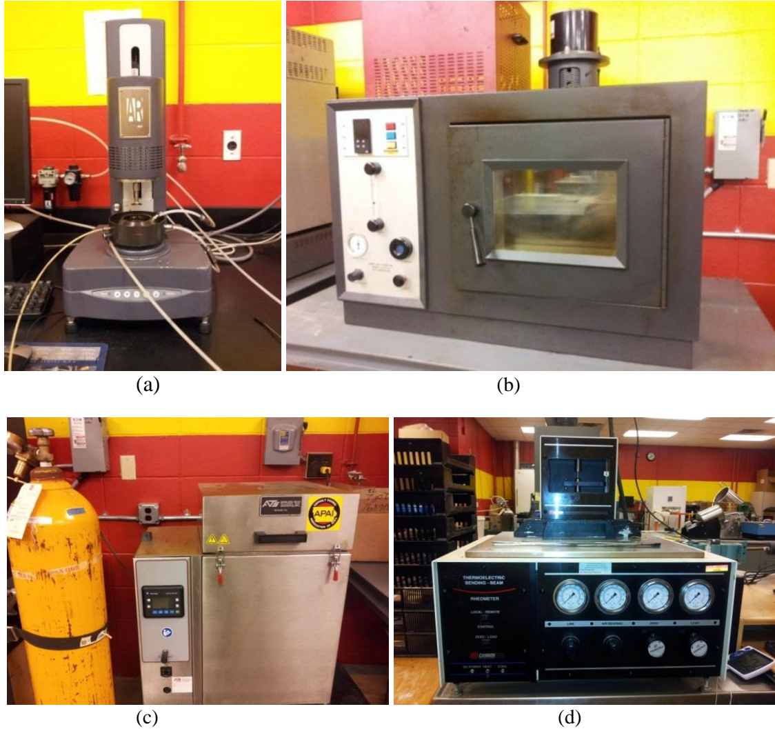
Figure 3.11 Binder testing equipment (a) Dynamic shear rheometer (b) Rolling thin film oven (c) Pressure aging vessel (d) Bending beam rheometer
