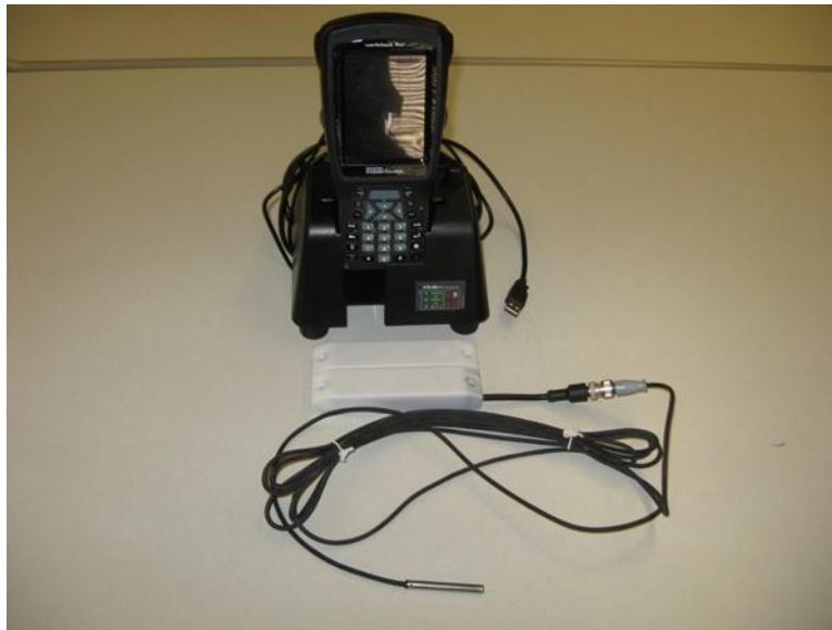
Figure 3-5. RFID tag and portable Pro.
