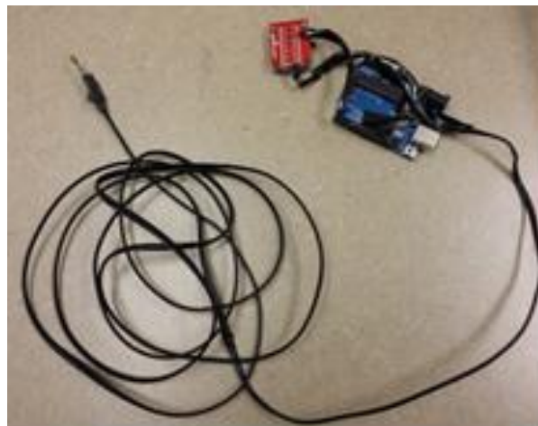
Figure 7: Wireless transmission end without batteries
