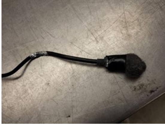
Figure 9: MEMS sensor with packaging
