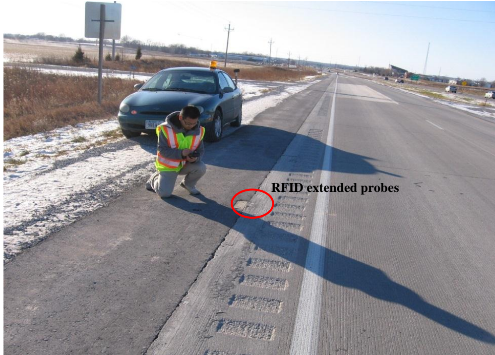
Figure 3-53. Data acquisition of RFID extended probes in winter.
