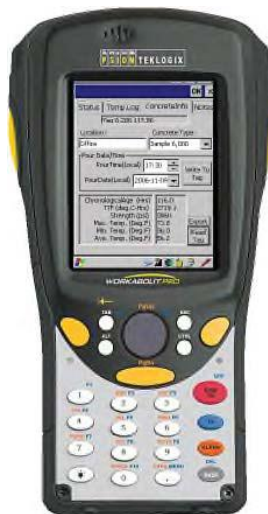
Figure 3-4. HardTrack portable handheld transceiver Pro (photo courtesy of WAKE, Inc.).
