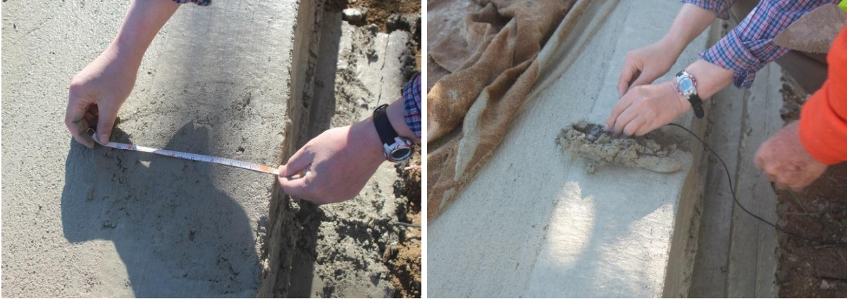
Figure 3-20. Embedment of MEMS digital humidity sensors.
