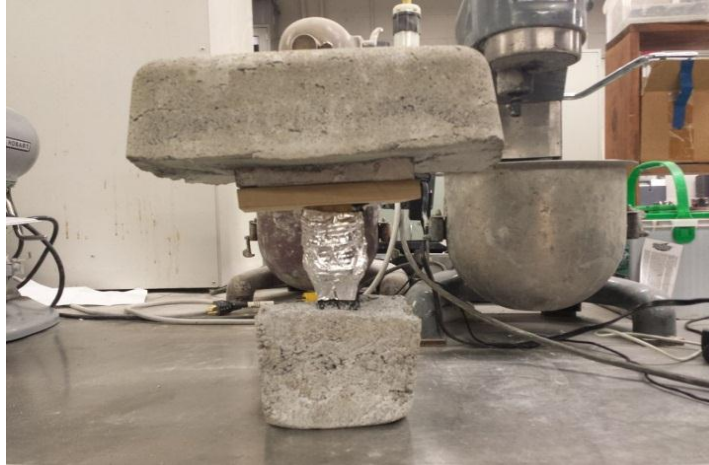
Figure 4-8. Wireless MEMS system inside concrete.
