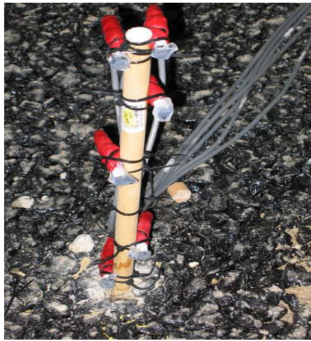
Figure 5-6. Moisture sensor packaging (Wells, 2005).
