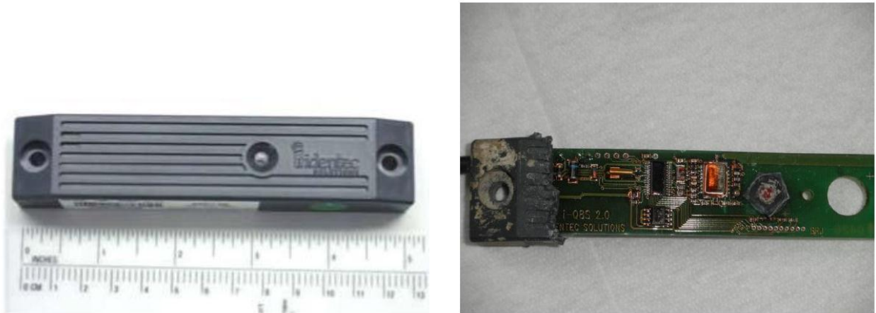
Figure 3-3. i-Q32T wireless RFID transponder (photo courtesy of WAKE, Inc.).
