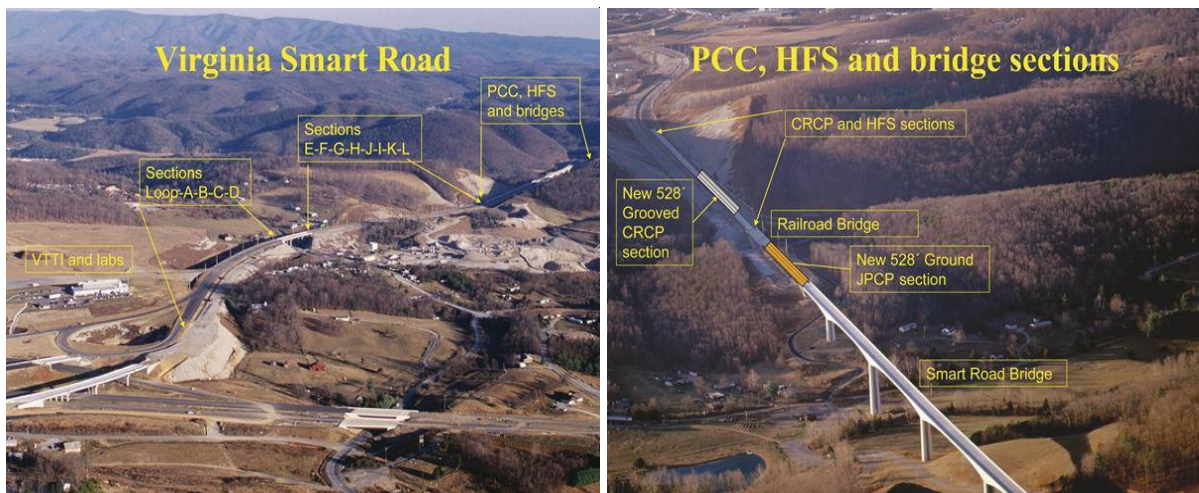
Figure 2-3. Virginia Smart Road (photo courtesy of Dr. Edgar de Leon Izeppi, Virginia Transportation Institute).
