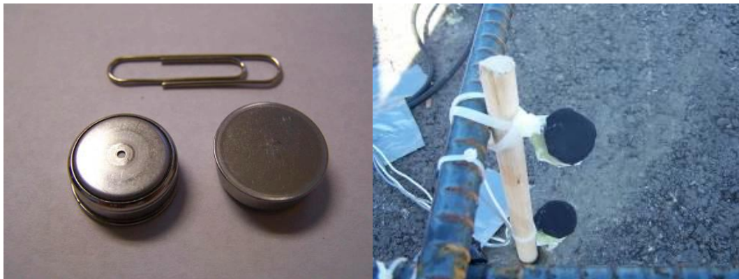
Figure 5-5. Hygrochron packaged in the field (Ye et al., 2006; Choi and Won, 2008).
