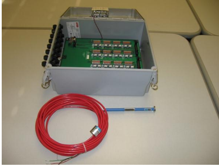
Figure 3-10. Datalogger and Model 4200 strain gage.
