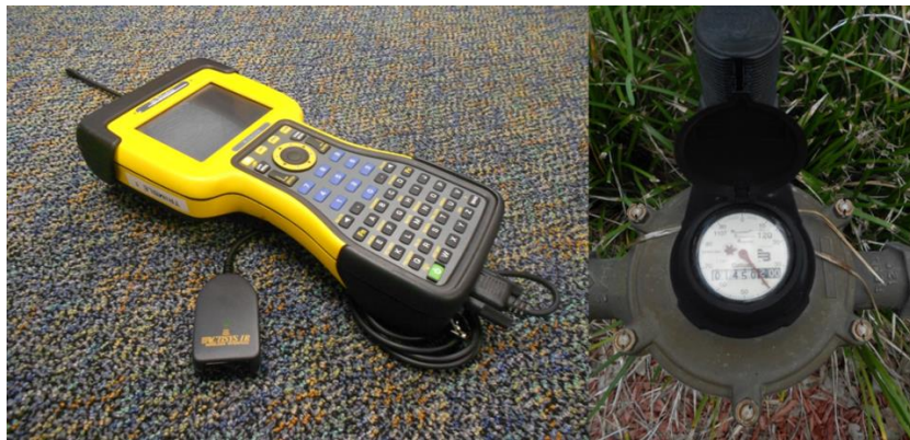
Figure 5.1: Transmitter used for water use data collection (left) and smart water meter (right).
