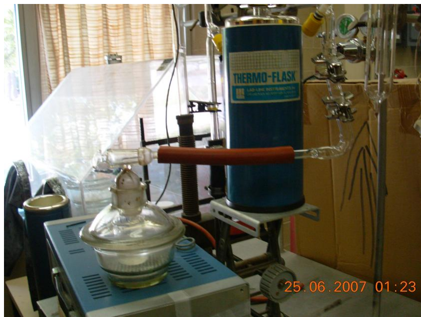
Figure 2.13: The pump system that saturates the sample. The beaker containing the sample is placed in the glass container on the picture.
