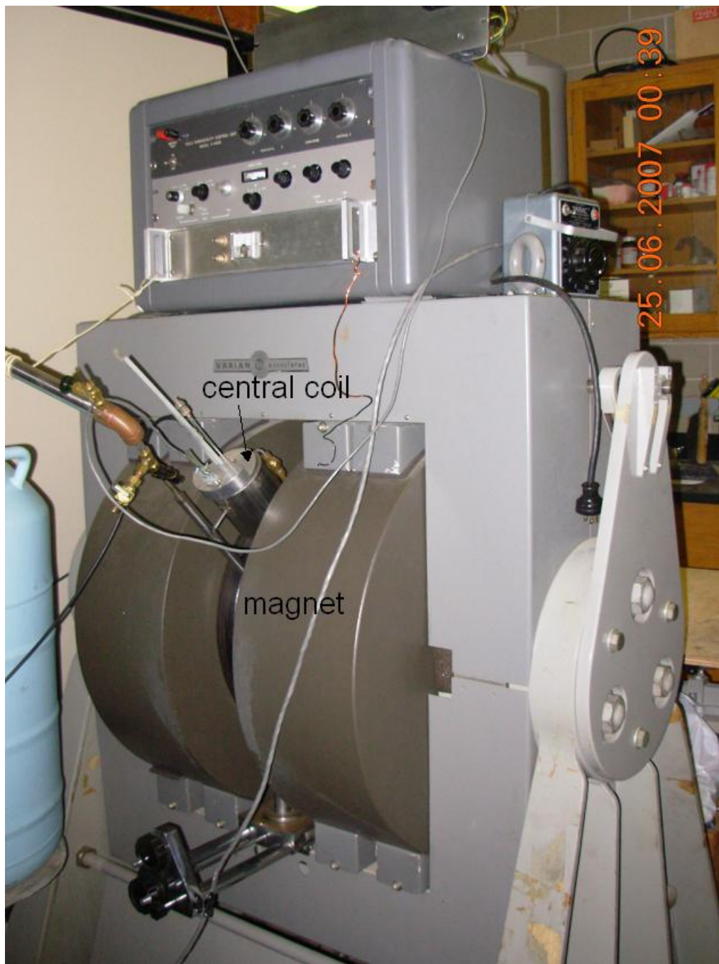
Figure 2.17: The 30 MHz NMR machine, housed in the UW Department of Physics building.
