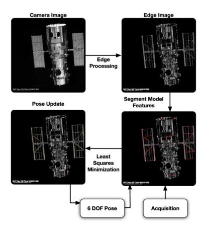
Figure 2.11: GNFIR Pose Process Loop [39]
