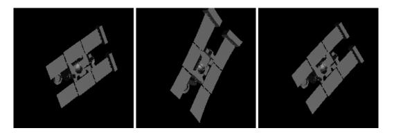
Figure 4.11: Undistorted image (left), radially distorted image (center), tangentially distorted (right)
