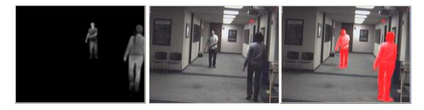
Figure 2.8: Infrared image (left), visible image (center), and human detection (right) [36]
