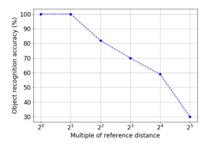
Figure 6.22: Recognition accuracy versus object distance
