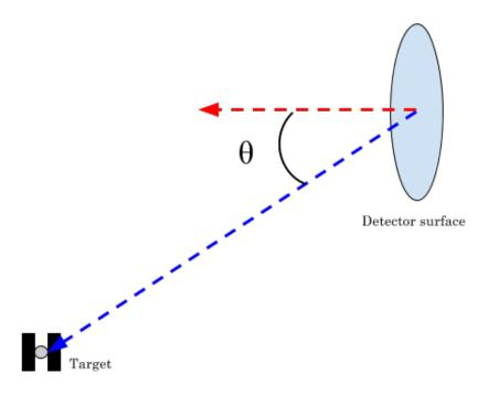
Figure 4.8: Line-of-sight angle ( $\theta$ ) definition for Equation 4.3
