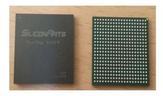
Figure 7.2: RayChip ray tracing chip [100]
