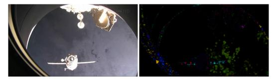
Figure 5.3: Dense optical flow segmentation (right) of Dragon docking (left)
