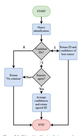
Figure 5.8: Object identification fusion procedure
