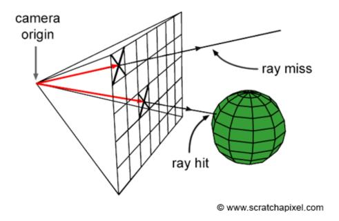
Figure 4.3: Ray-tracing for a basic scene [67]
