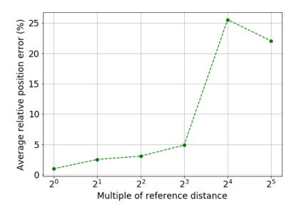
Figure 6.24: Relative position error versus object distance
