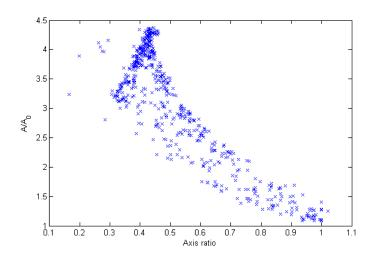
Figure 2.4: Example of projected area blobber distribution for a 3U CubeSat
