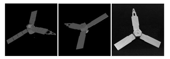
Figure 6.25: Original Juno model (left), modified model (center), and printed analog (right)
