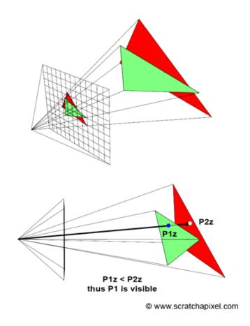
Figure 4.2: Z-buffer process with two differently colored triangles [65]
