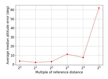
Figure 6.23: Average median attitude error versus object distance
