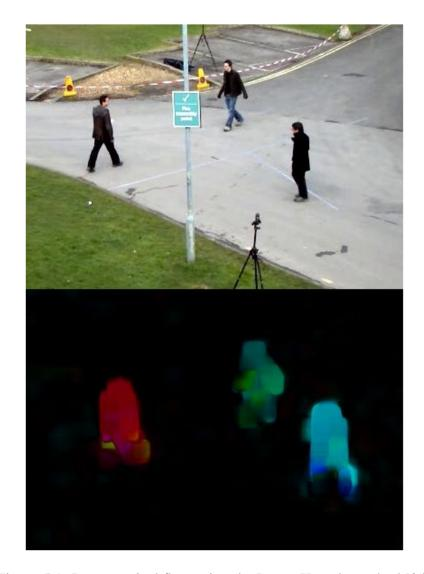
Figure 5.1: Dense optical flow using the Lucas-Kanade method [86]
