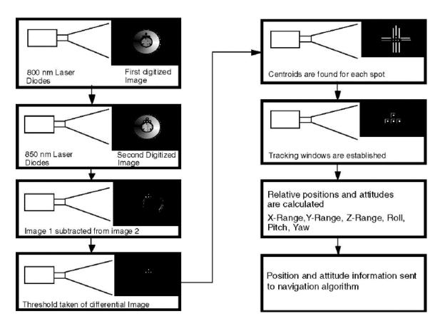
Figure 2.9: AVGS illumination and processing procedure [37]
