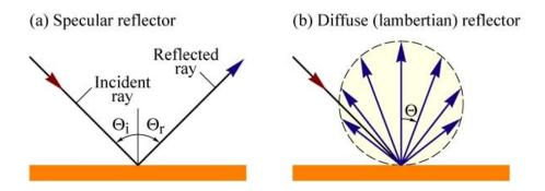
Figure 4.5: Specular (left) versus Lambertian (right) reflection [74]
