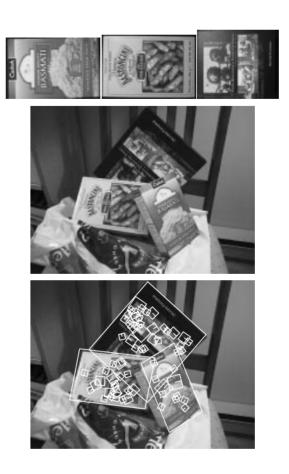
Figure 2.1: Model images of planar objects (top), test image (center), and recognition results showing model outlines and image keys used for matching (bottom) [12]
