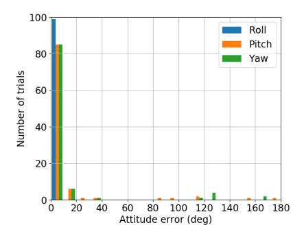
Figure 6.16: Fusion spectrum attitude error by axis
