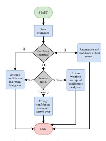
Figure 5.9: Pose estimation fusion procedure
