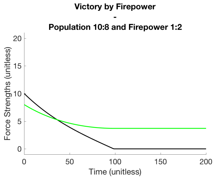
Figure 3.9: Illustration of Relative Firepower Dominating an Engagement Simulated by the Lanchester Equations
