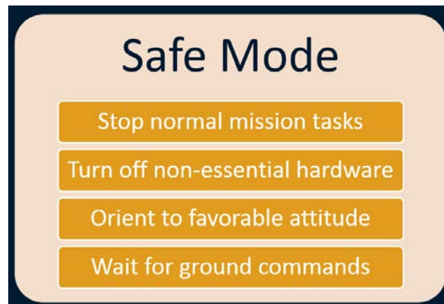
Figure 3 – Typical changes to spacecraft functionality during Safe Mode
