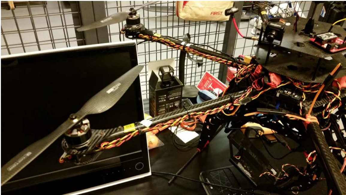
Figure 35 – Duplicate sensor suites installed on two adjacent UAV arms
