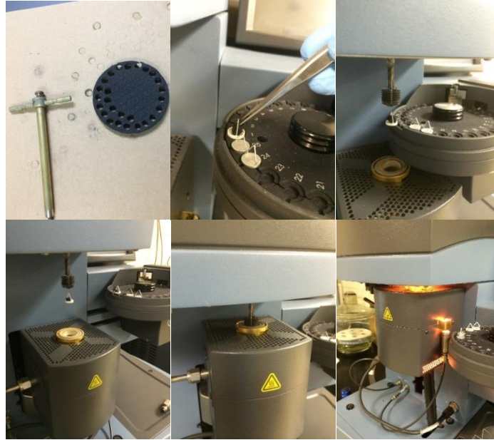
Figure 47: Sample Loading Procedure of KFA5 Samples into TA Q5000IR
