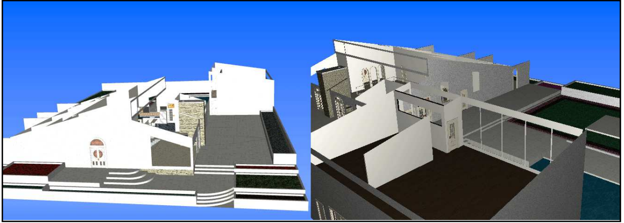
Figure 6.1: Abbreviated three-dimensional visualization of a house with JavaFX. The complete Wavefront model (obj file format) contains 781,000 vertices and faces; approximately 1/5th of the model is displayed [42, 65].
