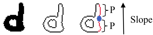
Figure 44: Handwritten letter contour and the slope calculation at each point (blue circle) per contour segment (red line).
