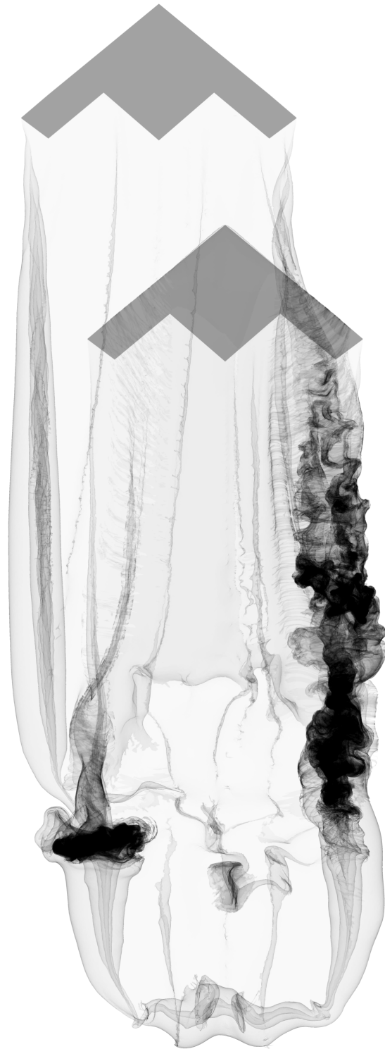
Figure 4.16: Shadowgraph of the simulated wakes. Darker regions indicate many layers of the vortex sheet.
