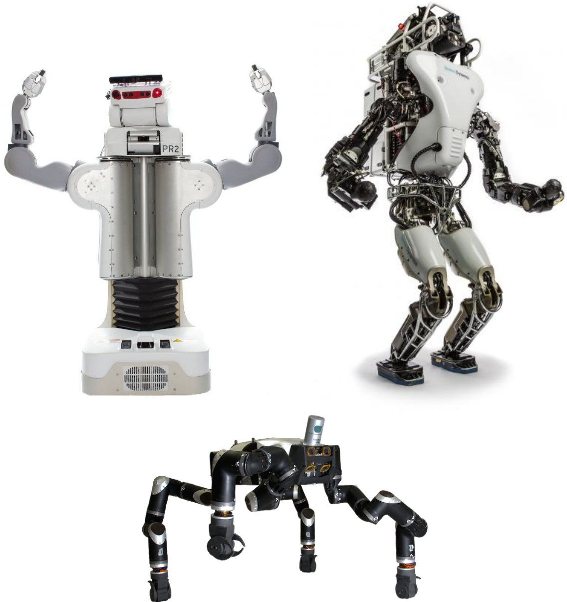
Figure 1.1: Robots with various mobility characteristics. Left: PR2 by Willow Garage, a traditional mobile manipulator. Right: Atlas by Boston Dynamics, a bipedal humanoid. Bottom: RoboSimian by NASA's Jet Propulsion Laboratory, a quadruped with wheels on its knees and feet.
