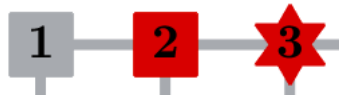
Figure 4.7: Tile number 1 is unused. Tile number 2 has a faulty Compute Resource. Tile number 3 has a faulty router.
