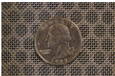
Figure 3.1: Metal mesh screen
