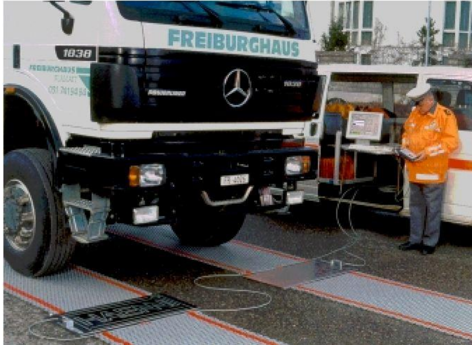
Figure 2-7: Capacitance mat WIM system connected with data acquisition devices. (Loadometer Corp, Baltimore)
