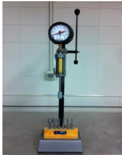
Figure 2. Device for penetration test
