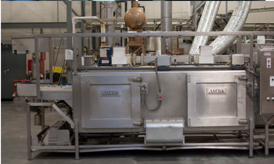
Microwave used for biomass drying provided by Cellencor
