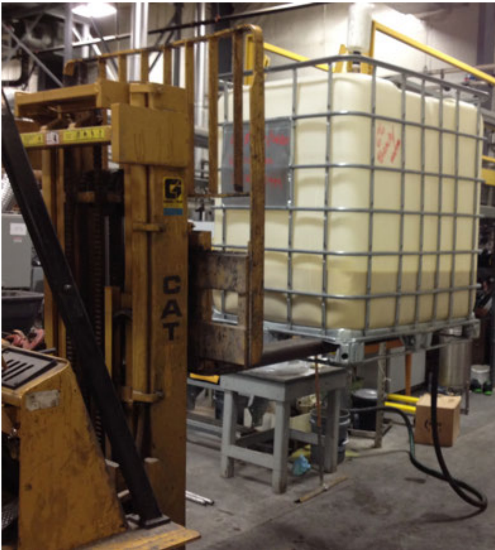
SV attached to pump to fill 1600L bioreactor, utilizing a fork lift to create head pressure. Notice filter on top of SV.
