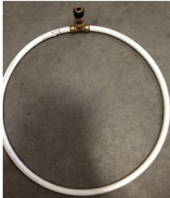
Column cooler (up to 2 of them)
