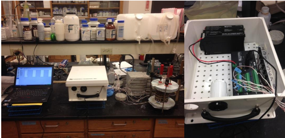
Figure 4.6 Data Acquisition System and Full Apparatus Setup for Cylindrical Specimen.
