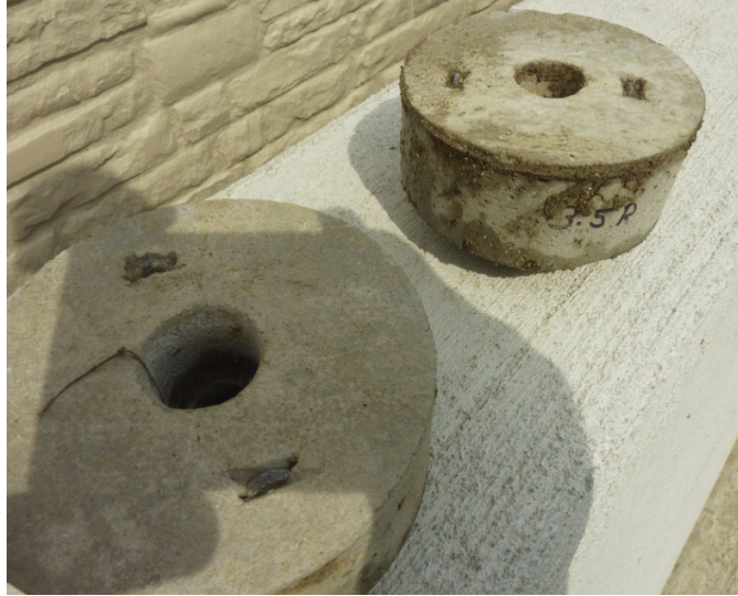
Figure 7.5. Coupon samples placed within TX Active test section.
