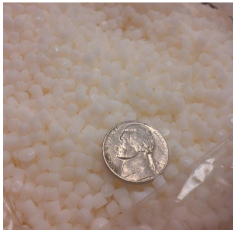
Figure 13. Polyoctenamer pellets 80% crystalline
