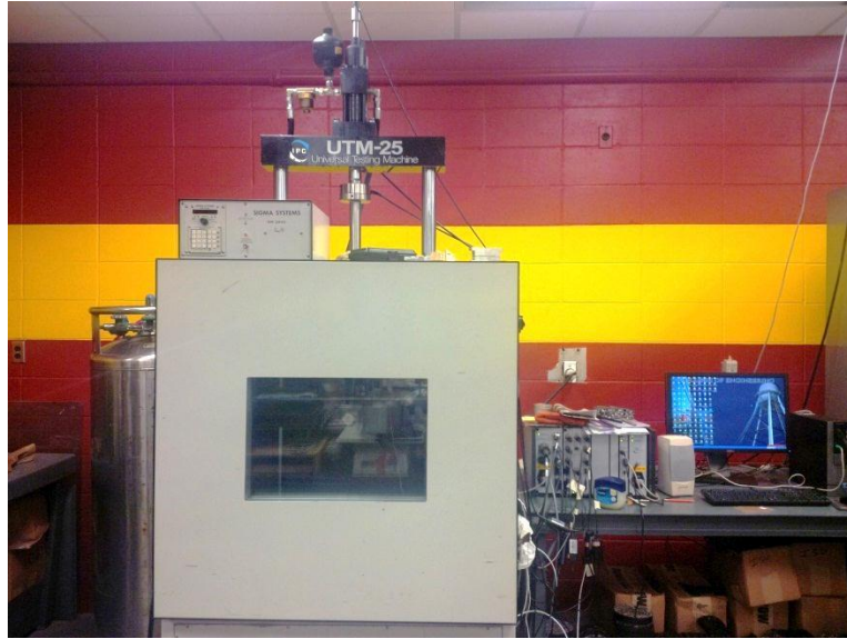
Figure 20. Universal testing machine (UTM-25) and data acquisition system
