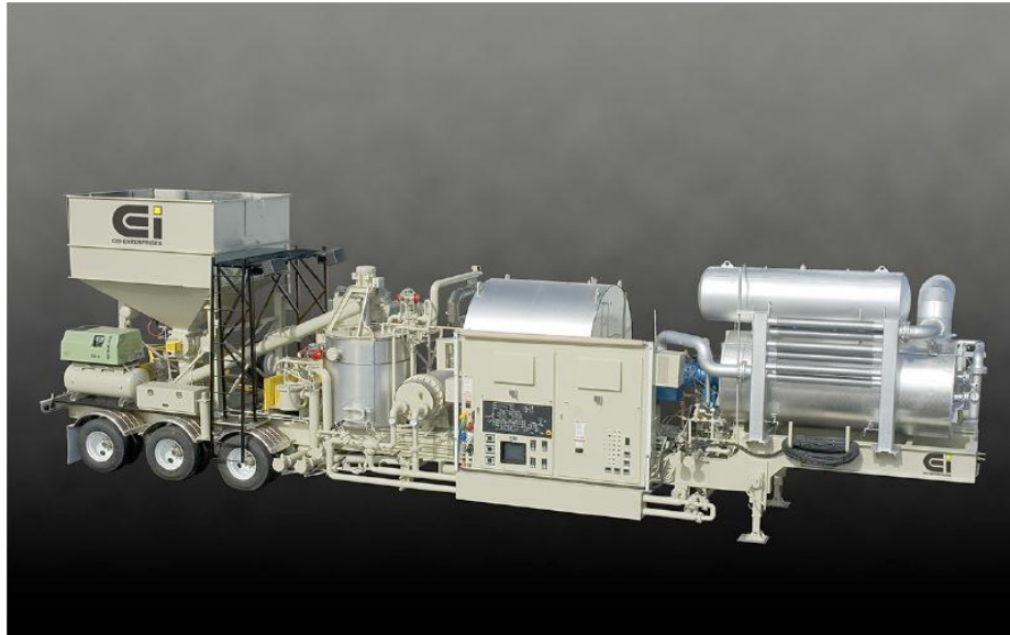
Figure 8. Example of on-site asphalt rubber blending plant (CEI Enterprises, 2008)
