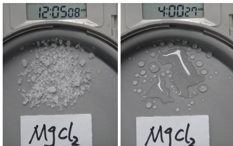
Figure 73. Melting of \text{MgCl}_2 by attracting water from atmosphere
