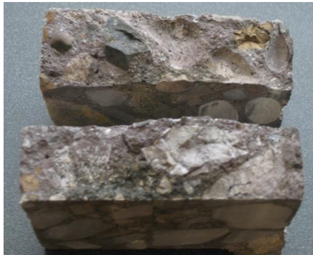
Figure 35. Fracture surface of silver nitrate sprayed samples
