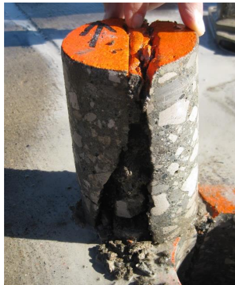
Figure 58. Core sample 4 from the distressed joint
