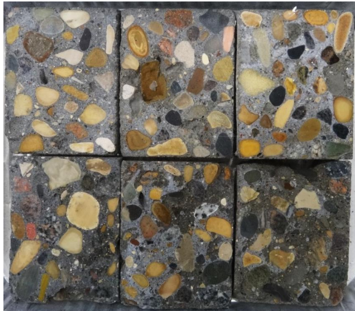
Figure 38. Sample exposed MgCl 2 solution during freezing and thawing (Top row: w/cm=0.38, bottom row: w/cm=0.45; left to right: silica fume contents are 10%, 5%, and 0%)
