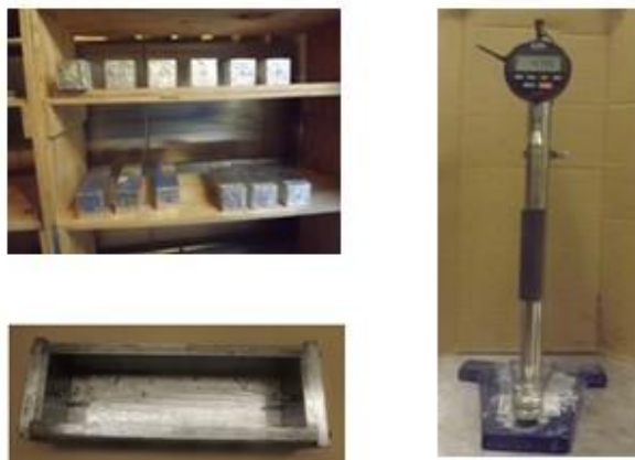
Figure 22 Mold, length comparator, and concrete specimens stored in the environment chamber
