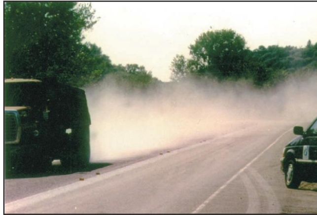
Figure 30: Dusty Aggregate Chip Seal (Wood et. al. 2006)
