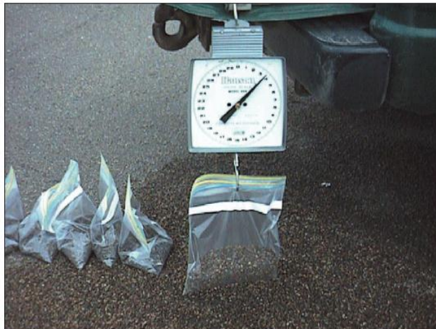
Figure 24: Chip Weighing (Wood et. al. 2006)
