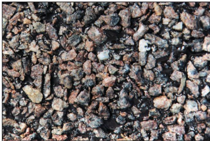
Figure 25: Correct Amount of Binder (Wood et. al. 2006)
