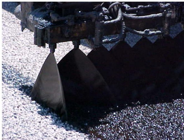
Figure 40: Inappropriate Nozzle Angle Alignment (MTAG 2007)
