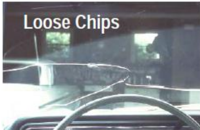
Figure 28: Windshield Damage Cause by Loose Chips (MTAG 2007)
