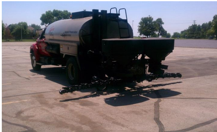
Figure 8: Distributor Truck with Sand Blotters (photo taken by author)
