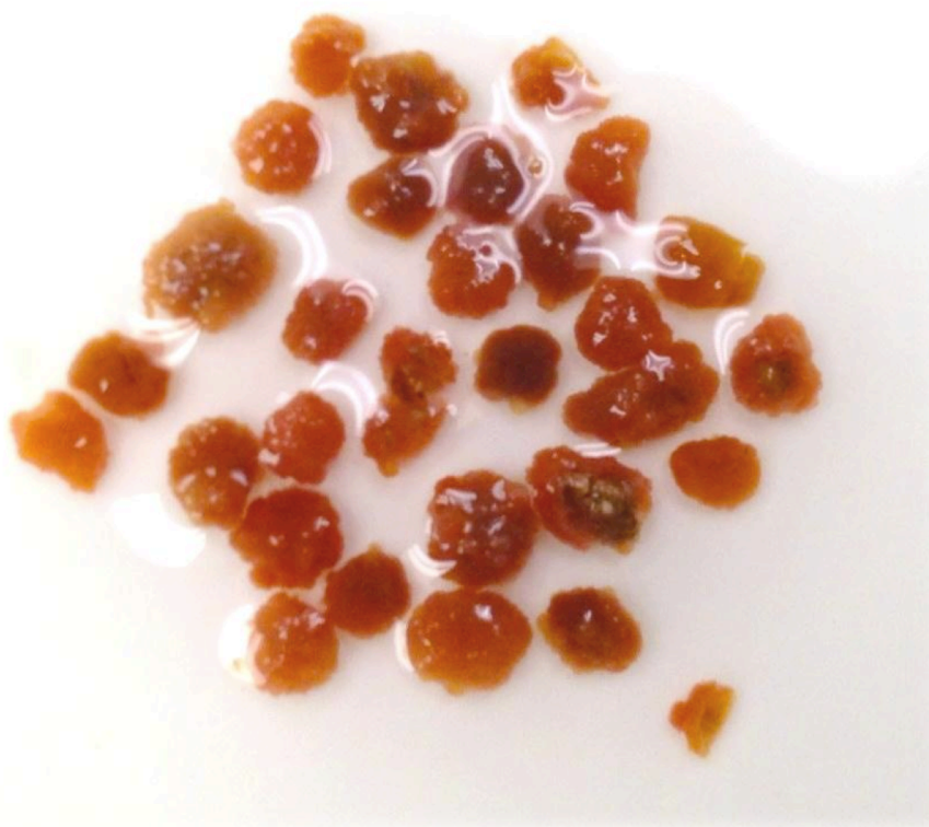
Fig. 7 Granules in UASB Anammox reactor (diameter approximately 3 mm)
