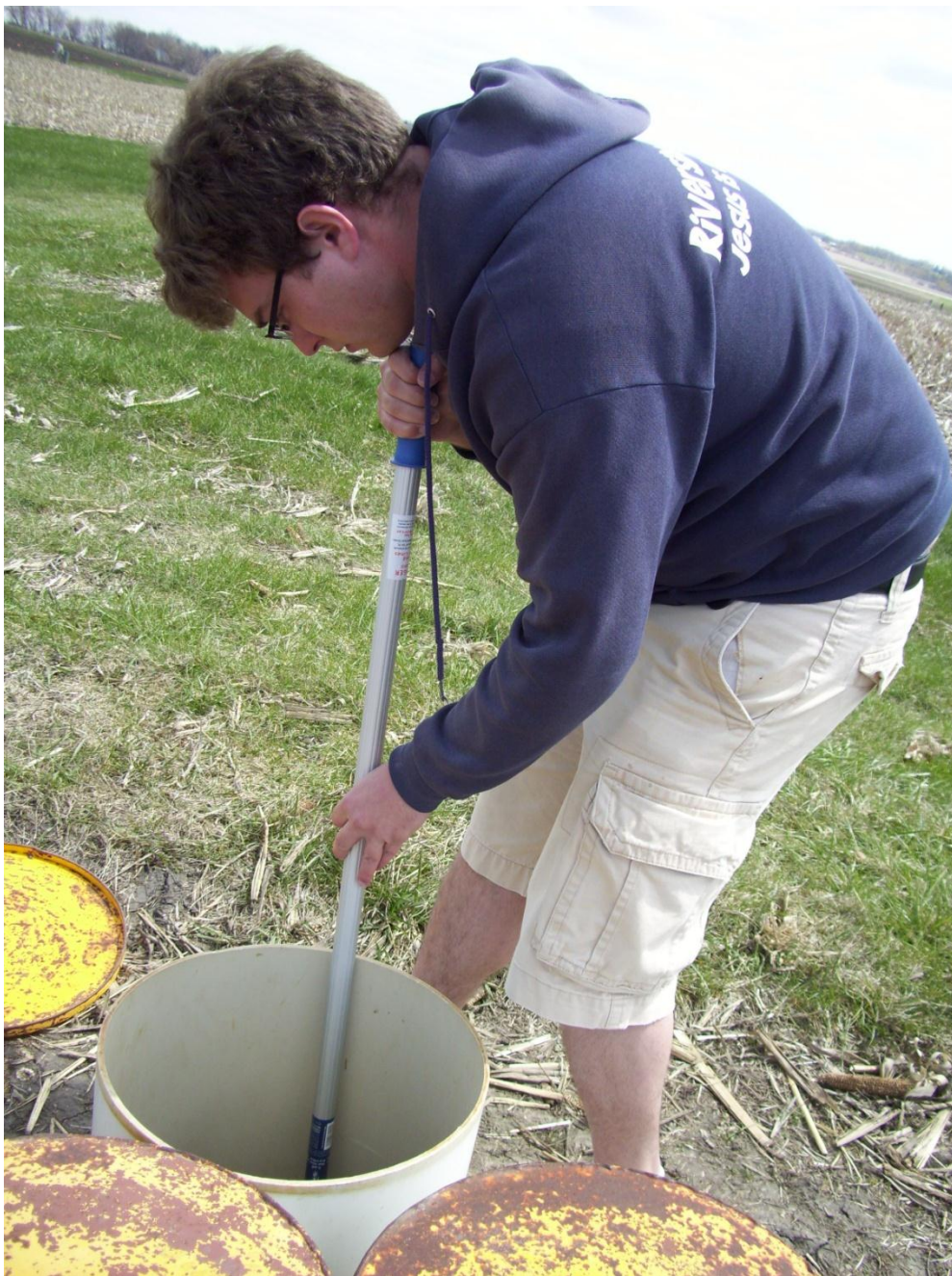
Figure 16: Tile water sample collection
