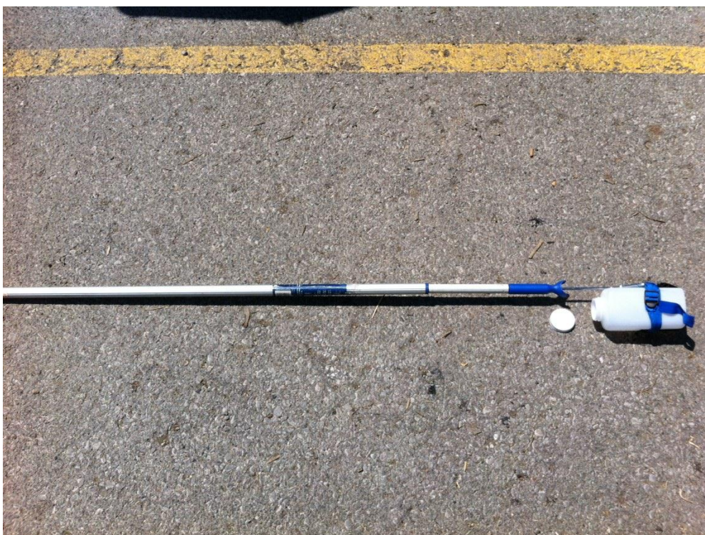
Figure 15: Tile water sample collection apparatus
