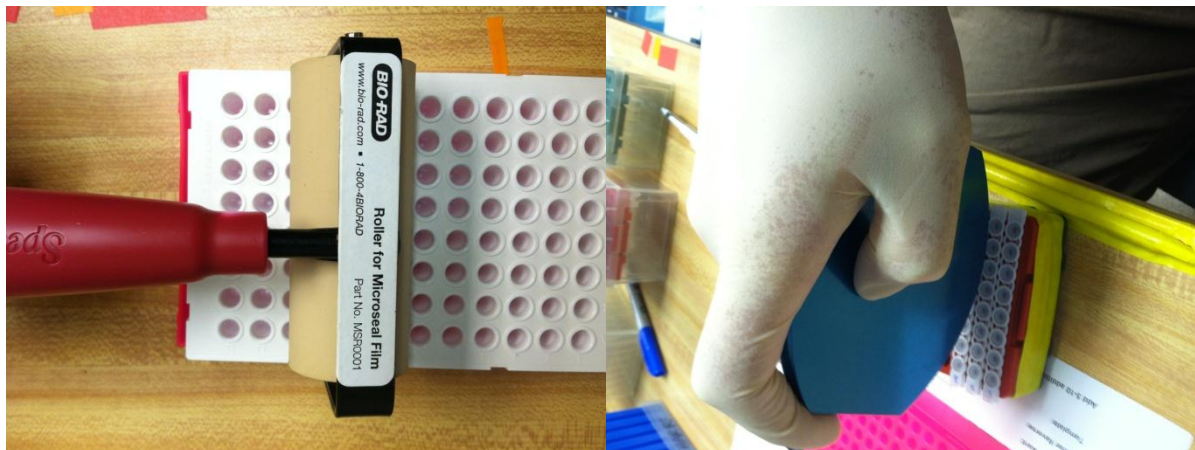
Figure 24: Roller (left) and capping tool (right) to seal plates or strips
