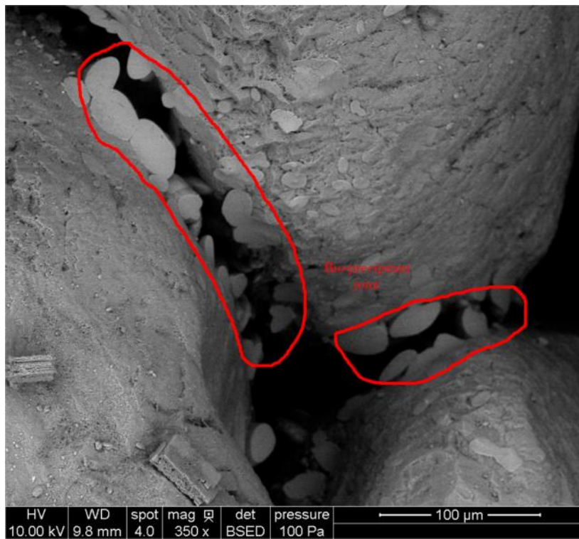
Figure 35. Silica sands with bio-treatment (350x)
