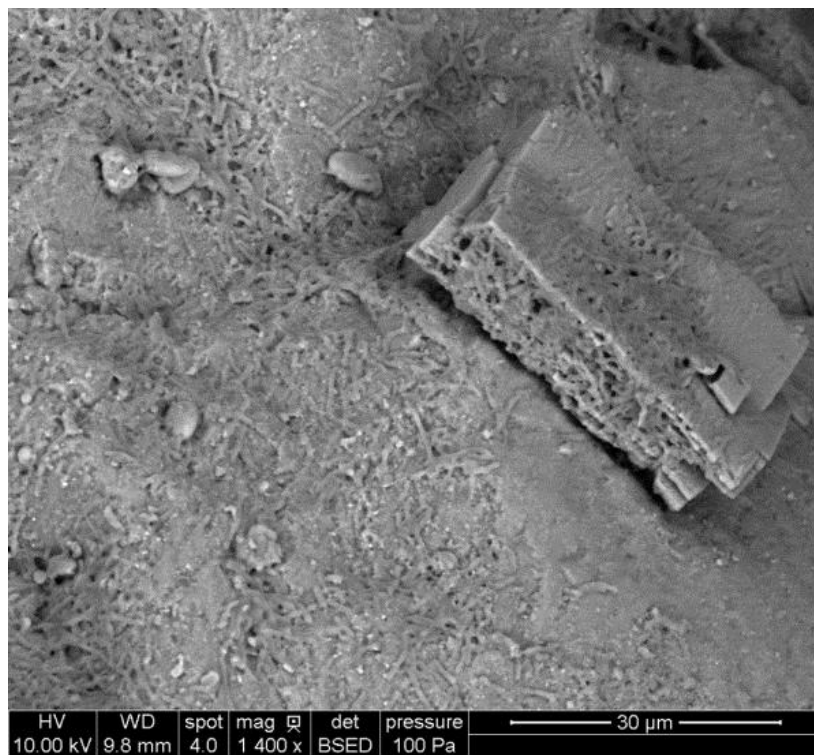
Figure 38. Silica sands with bio-treatment (1400x)
