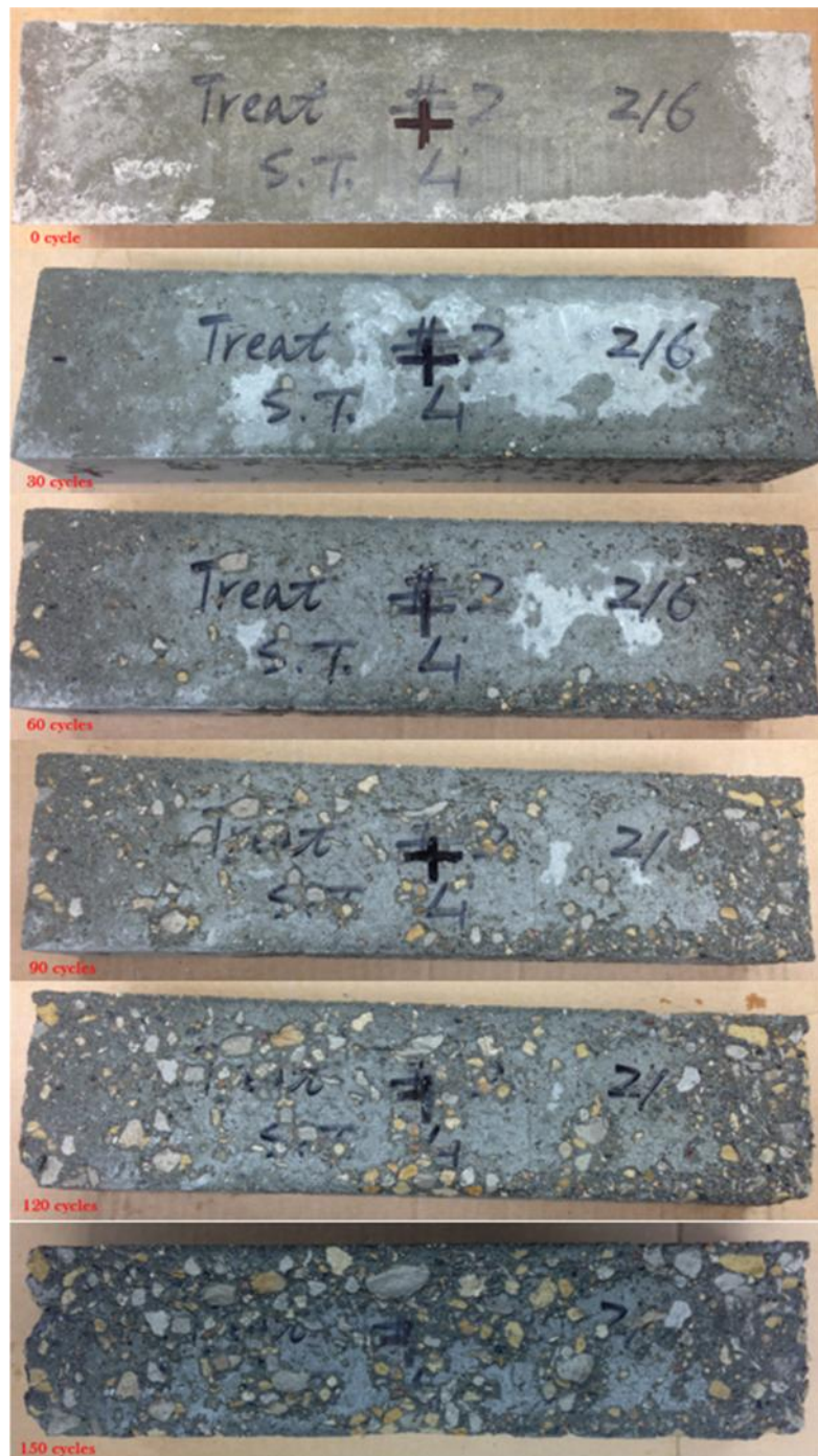
Figure 51. Bio-treated aggregate concrete beam at different freezing and thawing cycles
