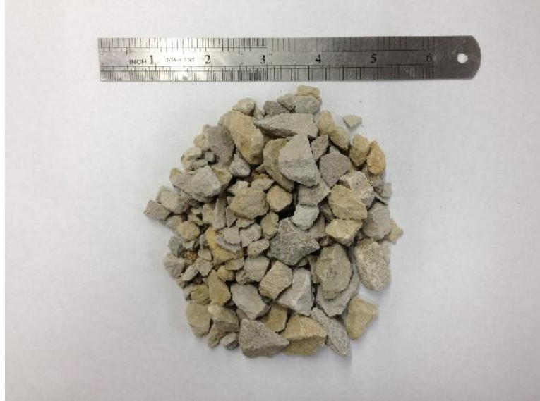
Figure 21. Concrete coarse aggregates without bio-treatment
