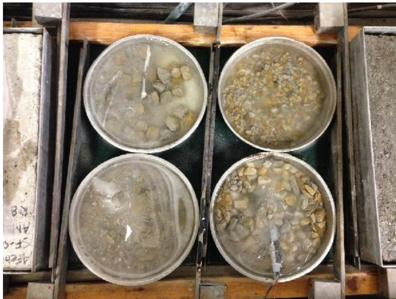
Figure 12. Soundness of aggregate testing in freeze-thaw cabinet
