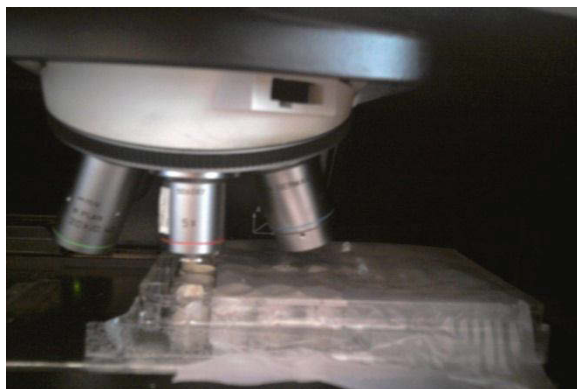
Figure 41: Typical setup of sample stored under the Raman microprobe
