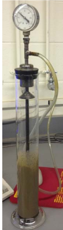
Figure 27. Air-jet dispersion tube use for mechanical agitation in ASTM D 422-63
