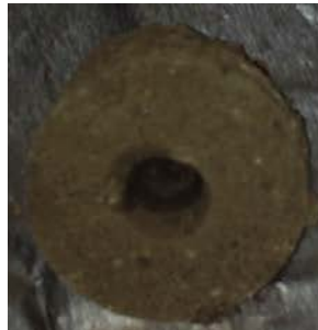
Figure 62. Aerial size of hole after pinhole test completion for alluvial top stratum
