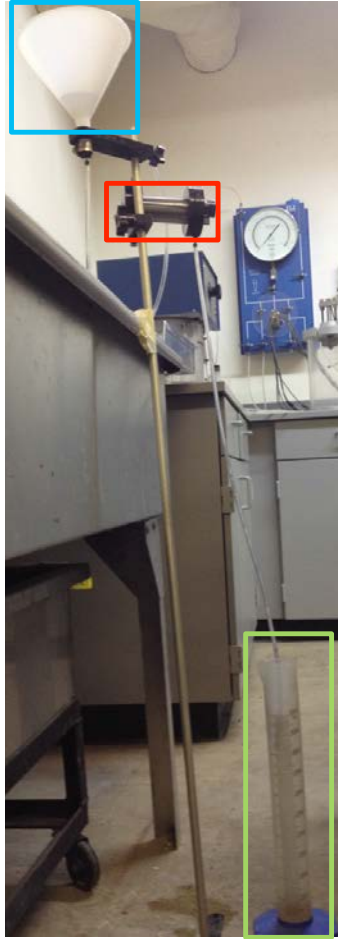
Figure 21. Complete assembled pinhole dispersion system
