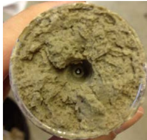
Figure 69. Aerial size of hole after pinhole test completion for Western Iowa loess
