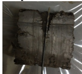
Figure 112. Inner size of hole compared with drill needle for treated sodium illite
