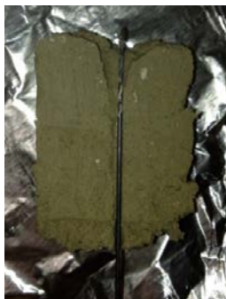
Figure 70. Inner size of hole compared with drill needle for Western Iowa loess
