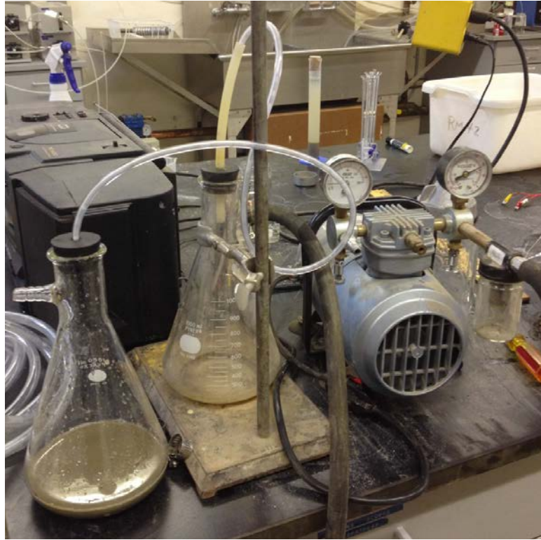
Figure 30. Vacuum used for de-airing of sample in ASTM D 4221-99
