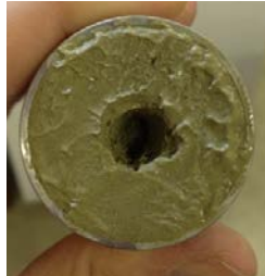
Figure 76. Aerial size of hole after pinhole test completion for untreated bentonite
