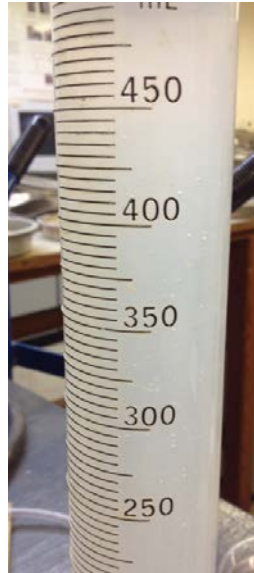
Figure 82. Effluent from pinhole test for treated bentonite
