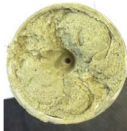
Figure 83. Aerial size of hole after pinhole test completion for treated bentonite
