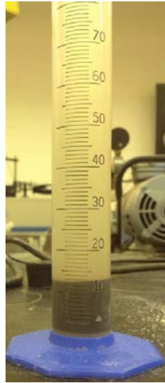
Figure 65. Final swell volume for modified free swell test for alluvial top stratum
