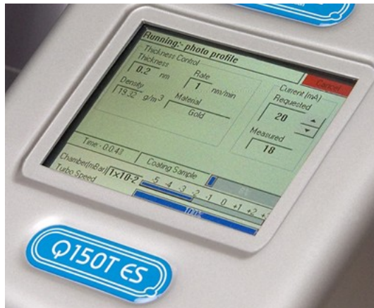
Figure 35. Touch screen control for Q150T sputter coater (Quorum Technologies, 2012)
