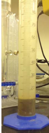
Figure 72. Final swell volume for modified free swell test for Western Iowa loess
