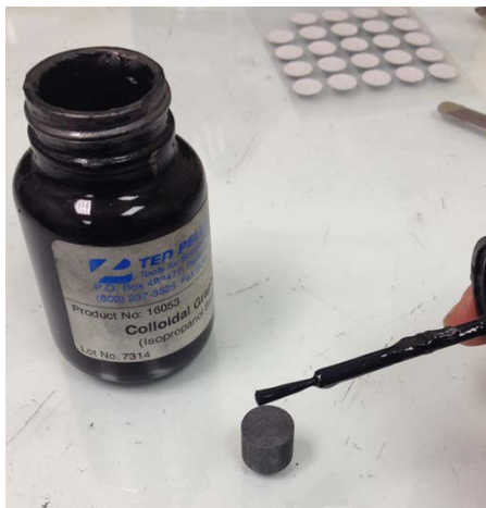
Figure 33. Graphite coating and brush used to affix soil sample to carbon stud
