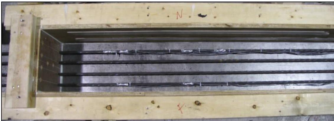
Figure 4-7: Instrumented Bottom Prestressing Strands in the Form
