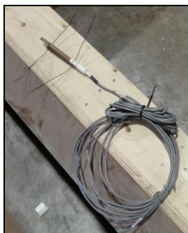
Figure 5-1: Embedded Concrete Strain Gage
