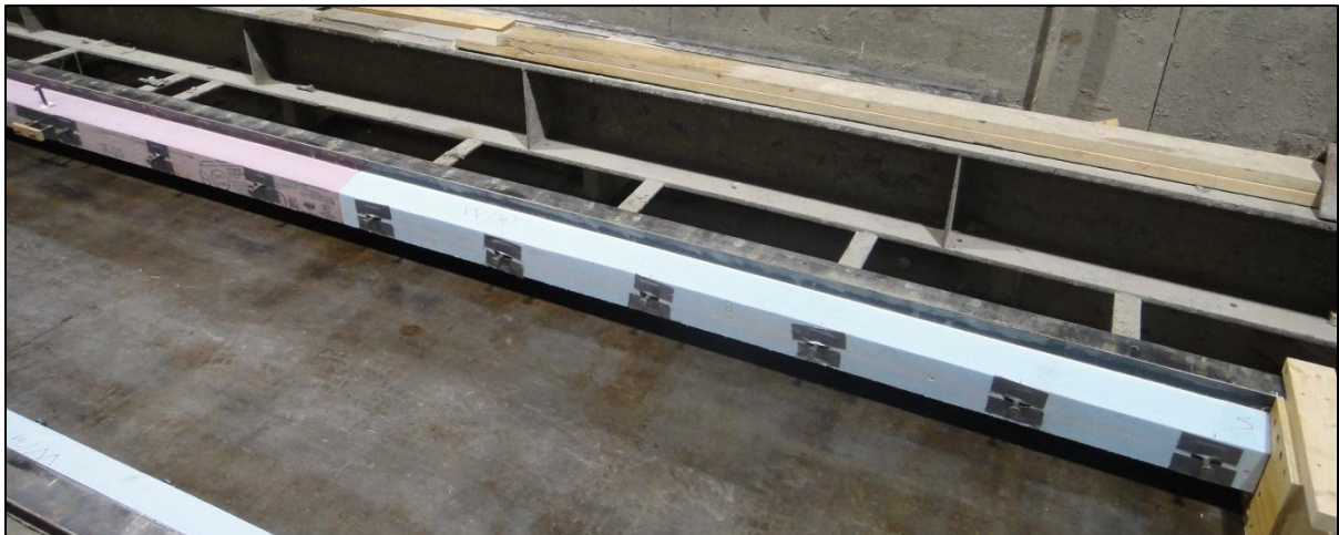
Figure 5-3: Locations of Steel Plates Embedded into P4
