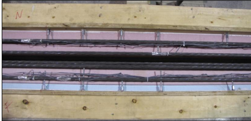
Figure 4-6: Location of Nuts to Fasten LVDTs
