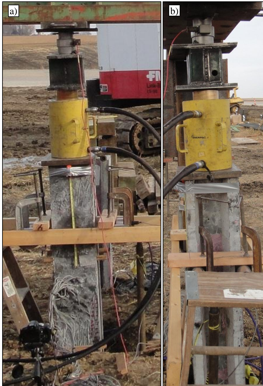
Figure 5-41: Tilt of P3 after Driving in the a) Weak-Axis Direction; and b) Strong-Axis Direction
