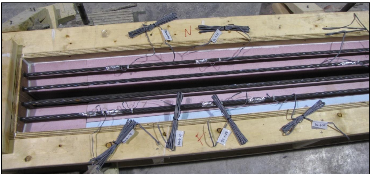
Figure D-1: TML Strain Gauge after the Aluminum Foil was Applied
