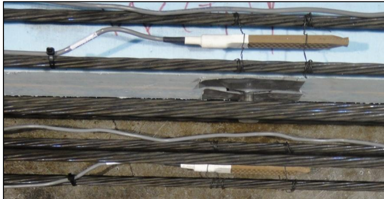
Figure D-3: Strung Embedded Concrete Strain Gage
