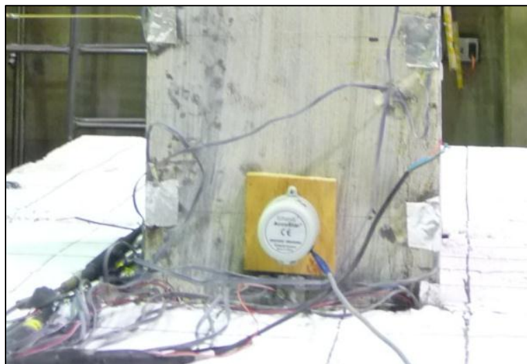
Figure 4-16: A Rotation Meter Attached to the Base of a Test Pile
