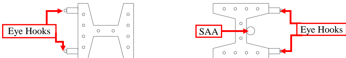
Figure 5-47: Illustration of Eye Hook and SAA Instrumentation Location
