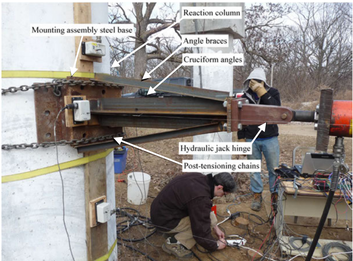
Figure 65. Steel assembly used to support the hydraulic jack.
