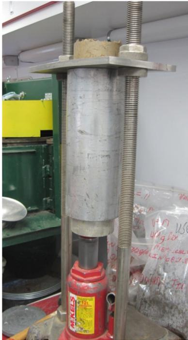
**Figure 13. Extruding a statically compacted specimen**
