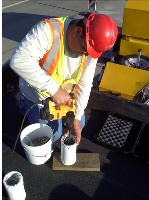
**Figure 20. Compaction of OGS+HDP sample in the field**
