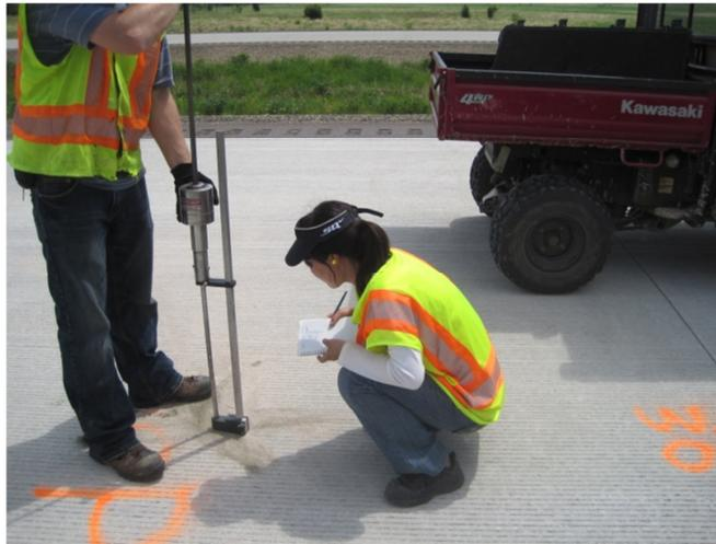
**Figure 4. A dynamic cone penetrometer (DCP) in use**
