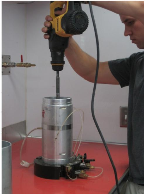
**Figure 15. Compaction of granular materials in split mold**
