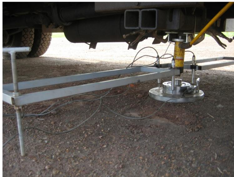
**Figure 5. Plate load test (PLT) performed on subgrade**
