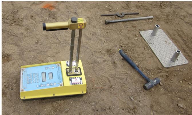
**Figure 28. Nuclear moisture-density gauge with auxiliary equipment**
