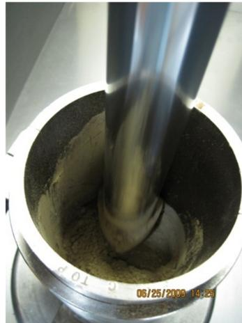
**Figure 9. Soil compacted by kneading tamper foot**
