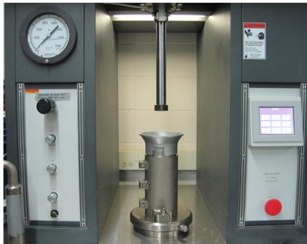
**Figure 8. Cox and Sons kneading compactor used for cohesive soils**
