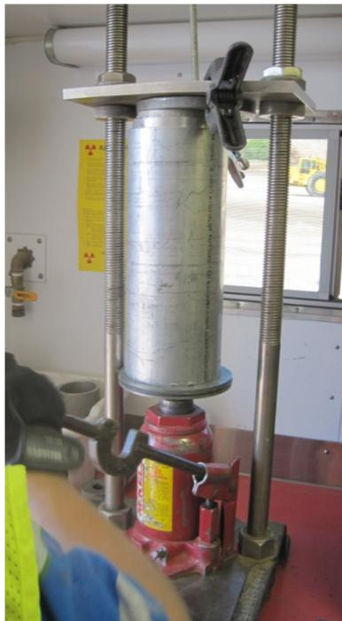
**Figure 12. Static compaction of a cohesive specimen**
